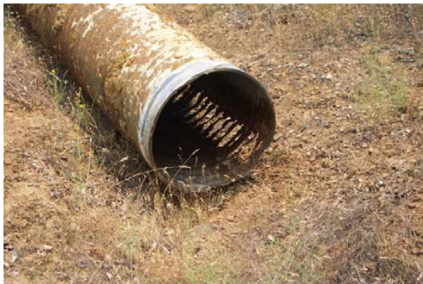
A rotted culvert removed on Indian Creek Road
